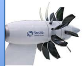
Geared drive counter rotating open rotor
