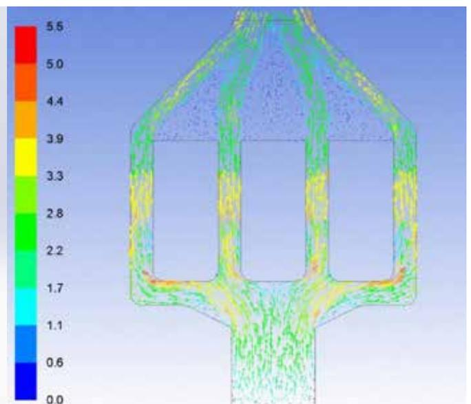
Simulation velocity vectors for the duct distributing air to four heat sinks
