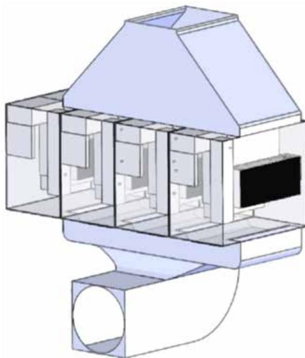
Power management bay cooling air duct assembly concept model
